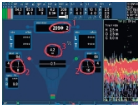
The haul is going on during a strong current with the towing direction. (1) GPS 4.9 knots, (2) TS 2.9 knots. This results in unstable doors (3) but double trawl and the gear hard in the bottom results in sustained contact with the bottom.
