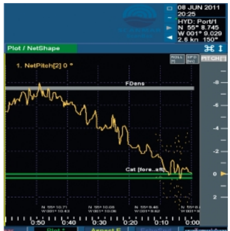
The filling indicator shows how the filling grade increases and the registrations show the exact position of fish entry. With the same position for the sensor on the trawl, the filling grade will always have the same gradient. The data is stored and can be used again on future trips.
