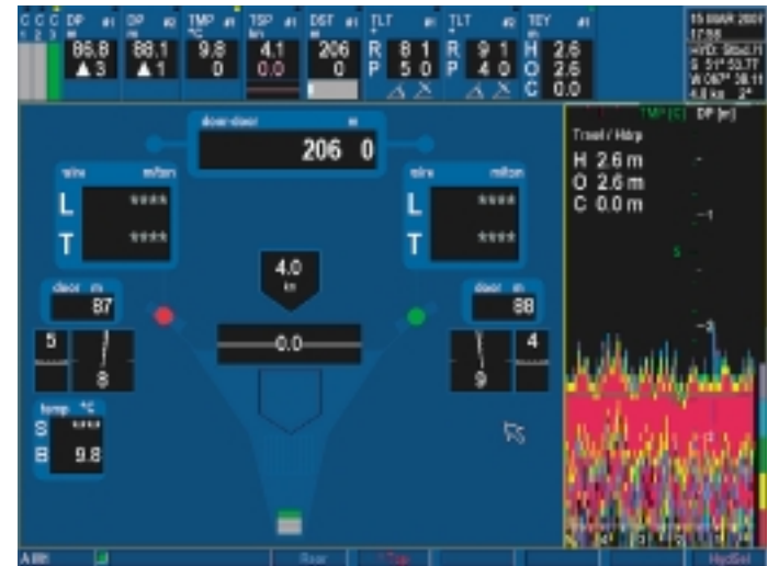
A screen capture from a ScanBas show's a «perfect» situation. With correct door angles (slightly inward leaning) and optimal towing speed for this bottom trawl, we see that the door distance is completely stable, the trawl is in symmetry, bottom gear has good contact and doors are totally stable. The result is optimal efficiency and lower fuel costs.
