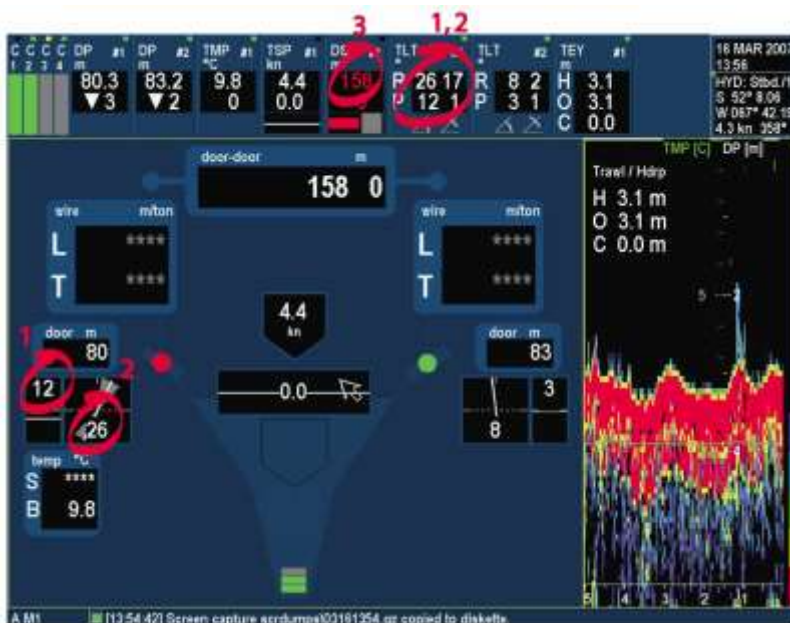
The port door loses bottom contact, the trawl collapses. (1+2) A lot of pitch and roll makes the door unstable and loses bottom contact. (3) the trawl doors lay down and lose contact.
