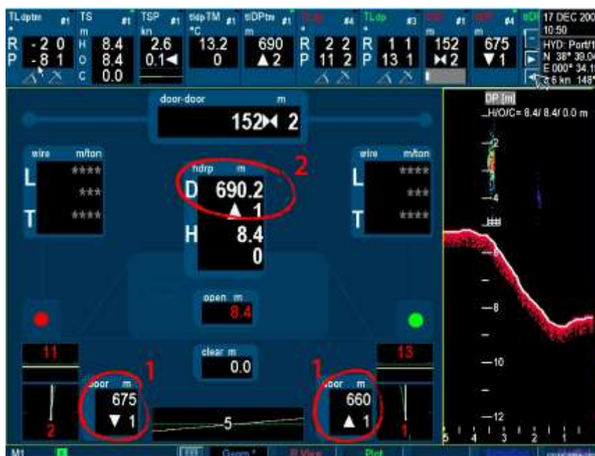
Trawling on edge: (1) the trawl doors on separate ridges depths 675 and 660 meters (2) in between the trawl 690 meters.
