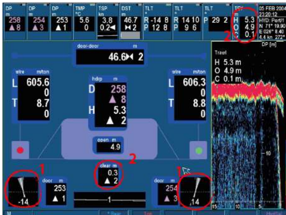
The trawl doors (1) have lost contact with the bottom and the trawl (2) is lifting.
